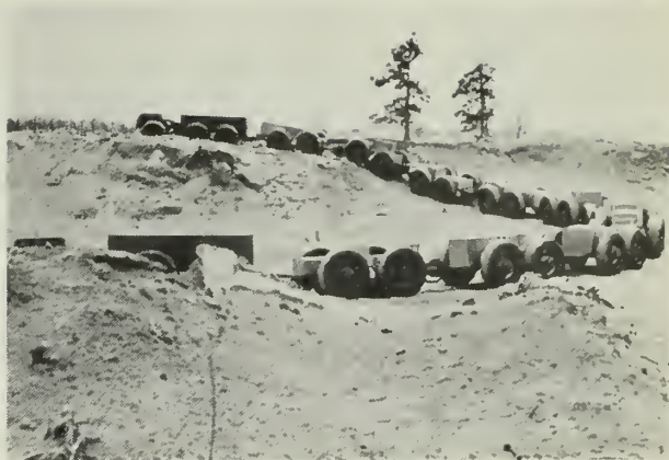
DERAILED—Train featuring 52-wheel drive is an Army overland cargo hauler that will track with precision.
